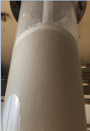
Fig.7 Schematic diagram of dust accumulation on top of the bed
