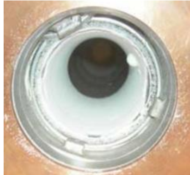
Polyethylene particles deposited on fluidized bed wall (view from bottom of bed)
