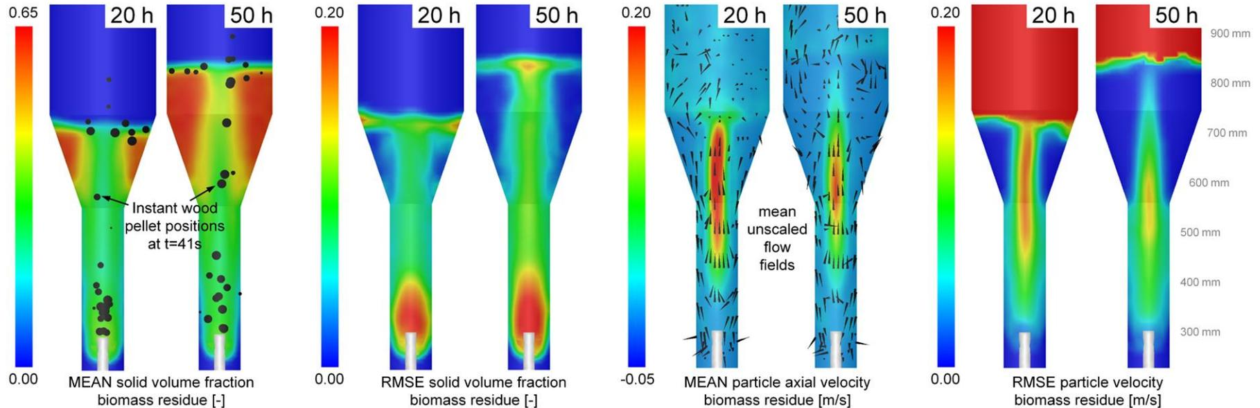
MEAN solid volume fraction distribution with RMSE values (left) and MEAN particle axial velocity with RMSE values (right) of the biomass residue at the center plane of the gasifier (averaged over 35 seconds).
