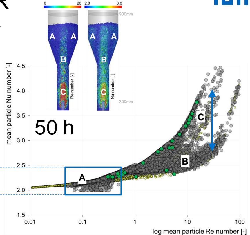
Mean particle Nu numbers of sand (yellow), biomass residue (gray), and wood pellets (green) over mean particle Re numbers (averaged over 35 seconds). *Heat transfer: Ranz-Marshall.*
