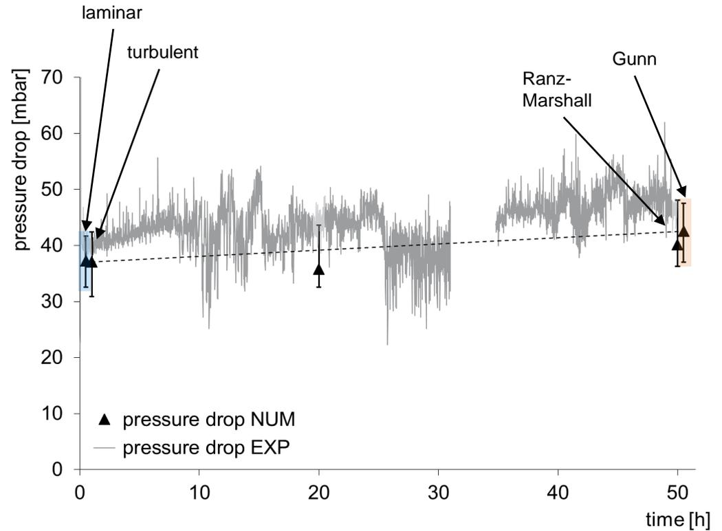
Numerical pressure drop for the start-up process (top) and after 50 h operational time (bottom).
