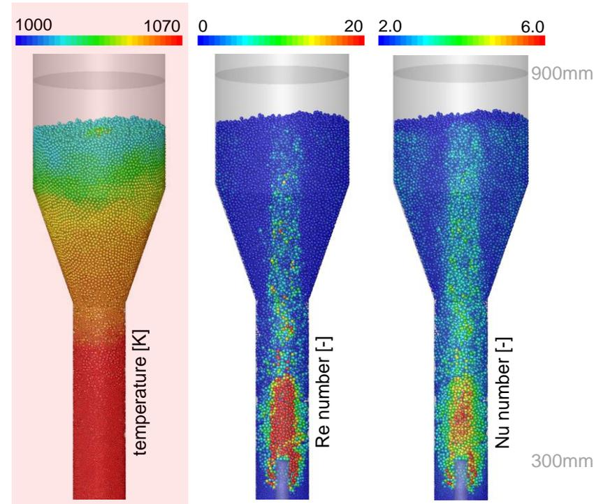
Particle temperature (left), as well as Re numbers (middle) and Nu numbers (right) after 41 seconds of simulation and a previous operating time of 50 hours.
