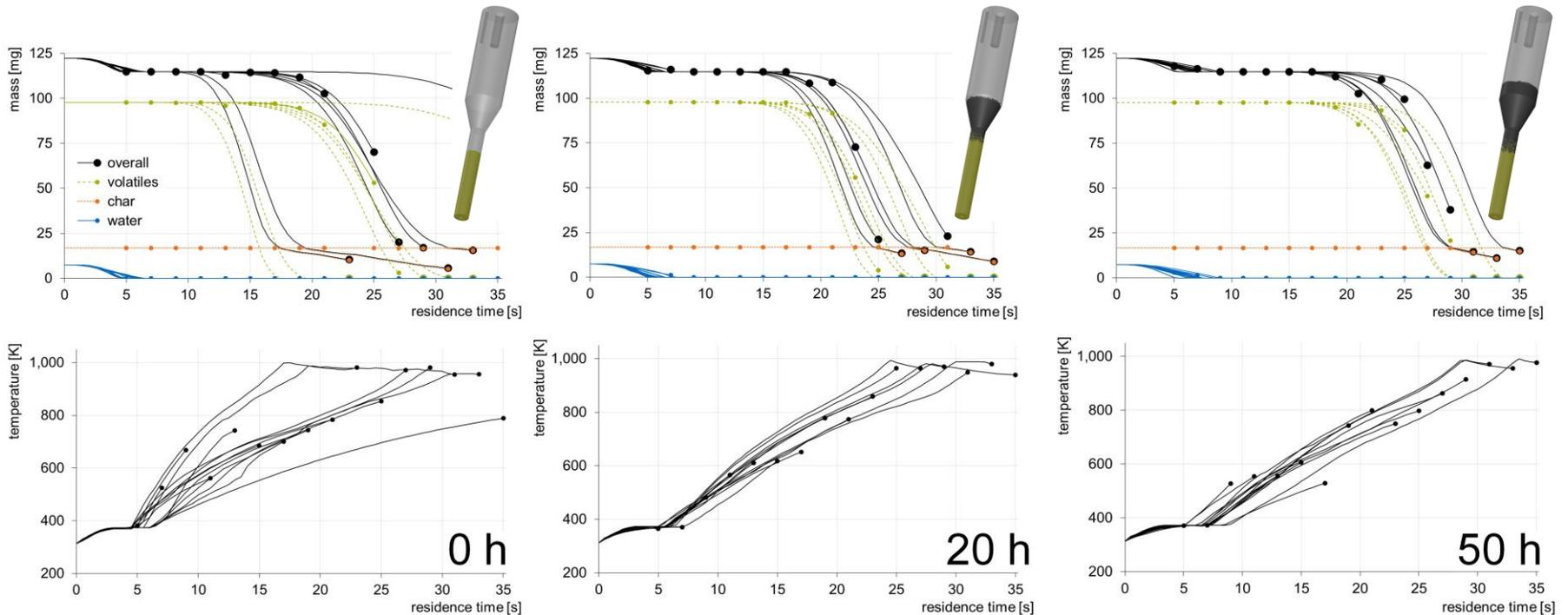
Evolution of composition (top) and temperature (bottom) of the biomass pellets injected between 6 and 36 seconds (residence times of at least 5 seconds). *Heat transfer: Ranz-Marshall.*
