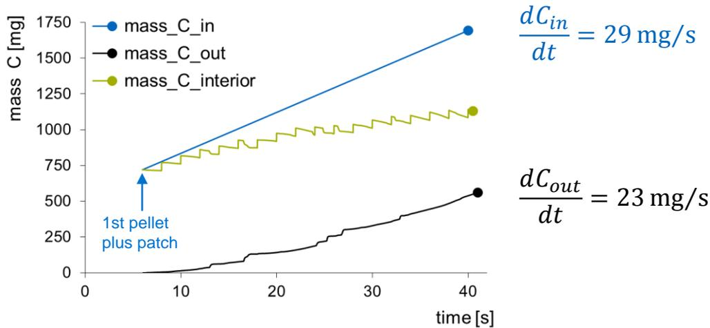
Mass of carbon into (blue) and out of the gasifier (black) and its accumulation inside (green) at 50 h.
