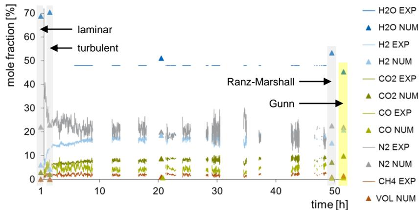
Numerical (symbols) and experimental (solid lines) product gas composition for different operating times.
