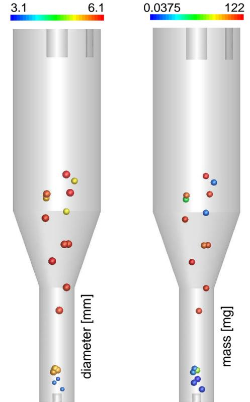
Diameter (left) and mass (right) of the wood pellets after 41 seconds of simulation at 50 h.
