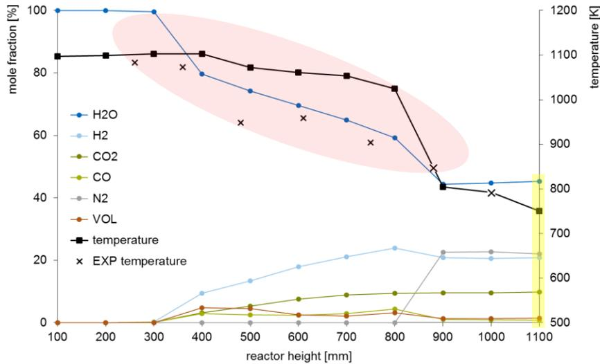
Cross-sectional-averaged numerical gas compositions, as well as experimental and numerical temperatures over the gasifier height.
