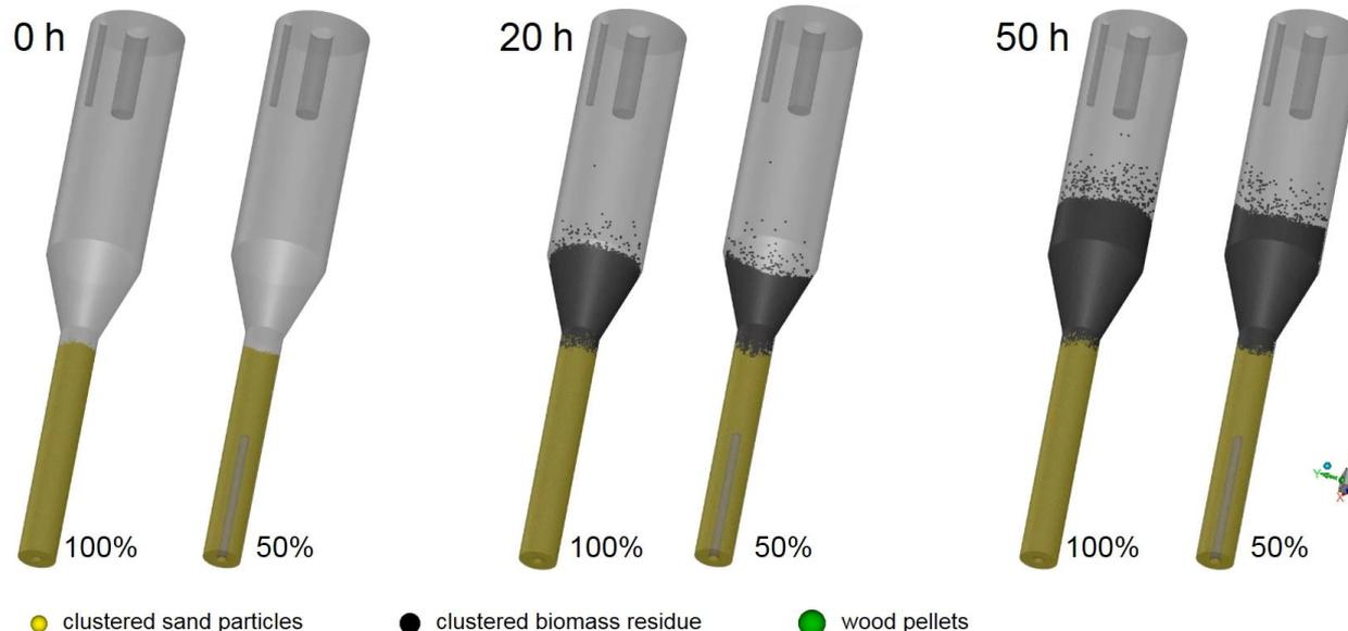
Fluidization behavior of inert sand particles (yellow), inert residue (black), and reactive wood pellets (green) for the start-up process/0h (left), after 20h (middle), and after 50h (right) operational time.
