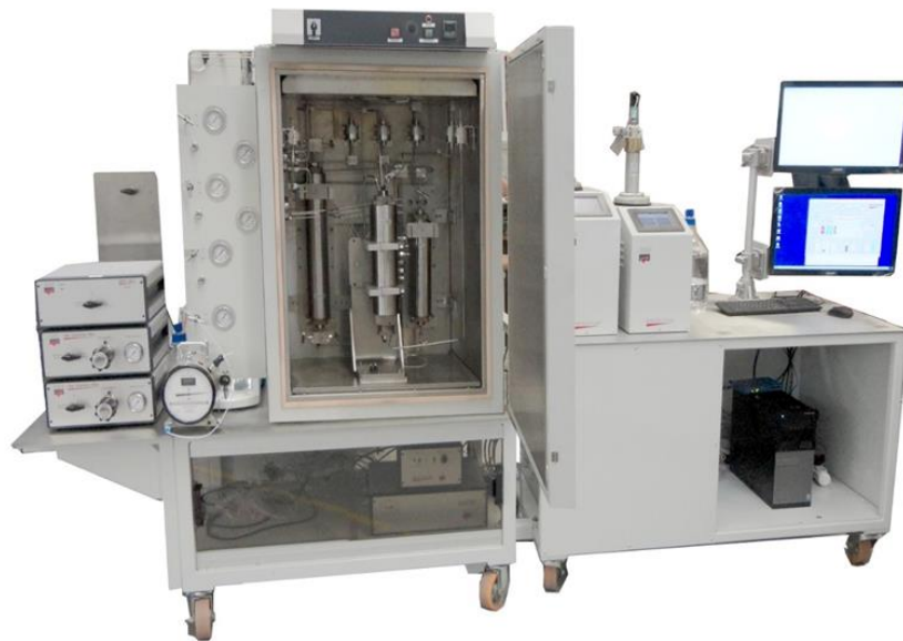
Fig. 1 Vinci core-flood system to be used for CO 2 injection in Bakken shale samples
