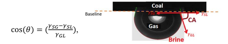
where  $\theta$  is the contact angle measured in the liquid,  $\gamma_{SG}$  is the gas/solid interfacial tension,  $\gamma_{SL}$  is the liquid/solid interfacial tension, and  $\gamma_{GL}$  is the gas/liquid interfacial tension.
