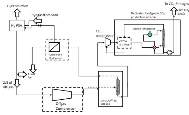
1st Carbon dioxide is removed by condensation
