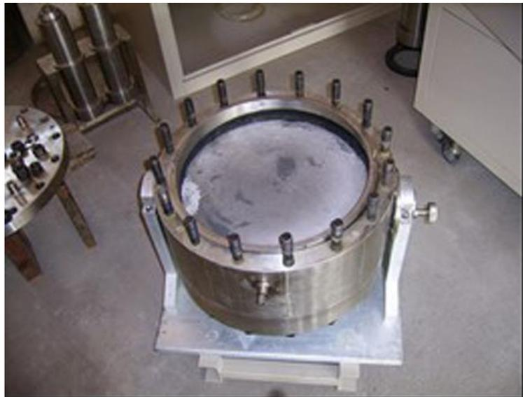
Fig.3 Coreholder of 3D physical model
