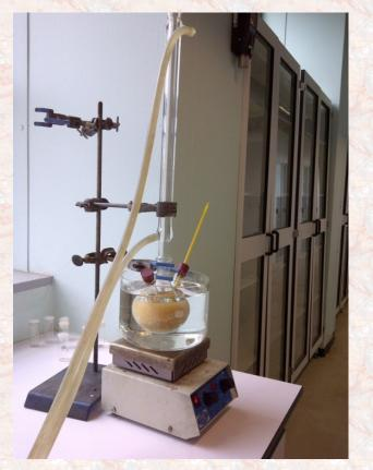
The equipment used in the transesterification setup is a Liebig condenser that is connected to a running tap.
