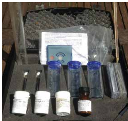
▲ Figure 2. A typical portable site analysis kit such as this one contains acidifying sewage effluent (SE) tablets, permanganate value tablets, universal pH tablets, sample containers, plastic test tubes, a turbidity tube, a test-tube brush, and a thermometer.
