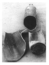
the failures of steel bolts during the construction of the eastern span of the San Francisco-Oakland Bay Bridge in 2013. While steel bolts serve as a prominent reference point, hydrogen embrittlement can be activated in most structural metal components exposed to hydrogen-producing environments.
