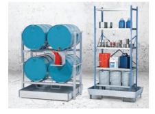
Pallet rack spill containment sumps are suitable for storing chemicals and highly corrosive liquids. The containment sumps can be positioned underneath drum racks to catch spills and drips from storage and dispensing. The sumps are constructed of galvanized heavy-gauge steel and feature a fully welded frame for durability and leak prevention. Forklift pockets allow for easy transport of the sumps. The sumps can also support vertical drum storage.
