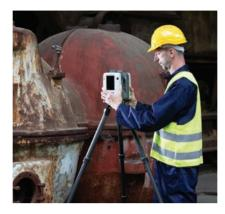
manufacturer's software to generate digital renderings. This technology is useful for industrial applications that require a digital model of a physical object or job site. The scanner provides models with excellent angular and range accuracy. **Artec**
