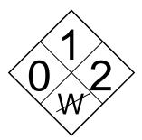
The area with a "0" in the diamond denotes health hazard, the area with the "1" denotes fire hazard and the area with a "2" denotes reactivity hazards. The box at the bottom is used to denote special hazards, e.g. incompatible with water.
