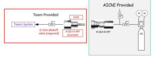
Example diagram showing what AIChE will provide for hydrogen delivery to a team. Also shown are the example fittings a team must provide.
