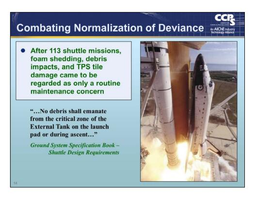
Early in the Shuttle Program, foam loss had been considered a dangerous problem. Design engineers were extremely concerned about potential damage to the Orbiter and the fragile TPS. The assumption that only tiny pieces of debris would strike the Orbiter was also built into original design requirements.
