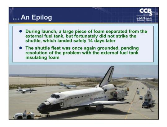
During the launch of Discovery, a large piece of insulating foam broke off of the external fuel tank but, fortuitously, did not strike the Orbiter.
