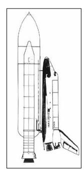
The leak from the booster rocket field joint continued to grow, impinging upon the lower portion of the external fuel tank. The external fuel tank contained (in separate vessels) the liquid hydrogen and liquid oxygen fuel that powered the shuttle's main engines. At about 65 seconds into the mission, the liquid hydrogen tank began to leak.
