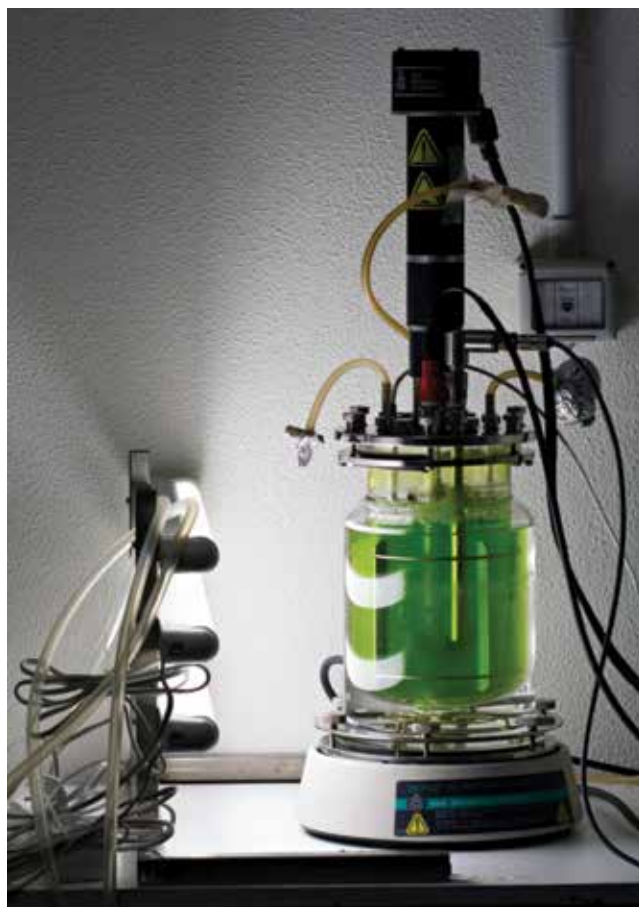
▲ Figure 6. Green algae in a fermentation bioreactor at the laboratory scale. Image courtesy of Umberto Salvagnin, Dept. of Sustainable Agro-Ecosystems and Bioresources, Centro Ricerca e Innovazione, Italy.
