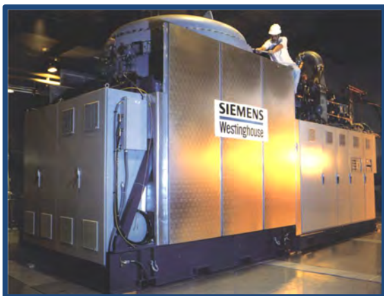
Siemens/Westinghouse 220 kWe Pressurized SOFC/GAS Turbine Hybrid System
