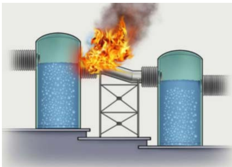
Figure 5.4. Flixborough temporary pipe illustration [42]
