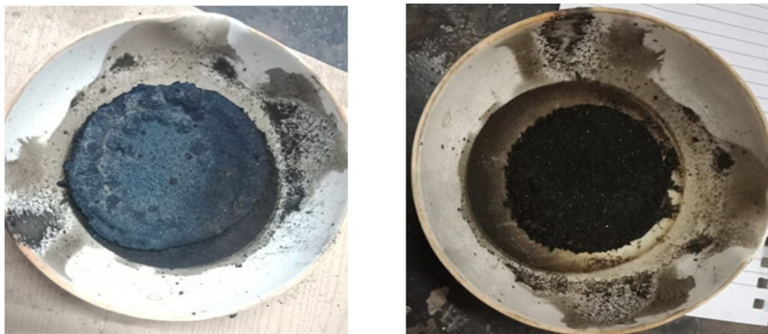
Figure 6. (A) GO coated Sand (After Annealing) and (B) GO Coated Sand (Crushed)
