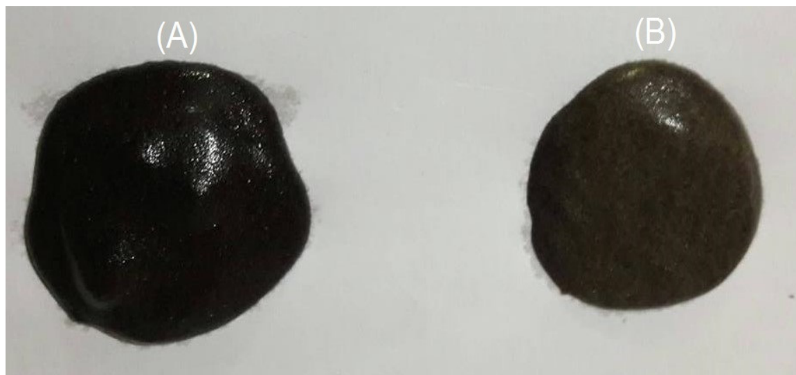
Figure 7 (A) Graphene Oxide Coated Sand Particles and (B) Washed River Sand
