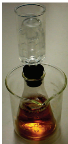
Figure 1: Brewing with Bioreactors DEMo uses bakers yeast and sugar to demonstrate the growth phases of single cell organisms in bioreactors. The Erlenmeyer flask set inside the beaker introduces the concept of a jacketed reactor. The airlock can introduce discussions about contamination and also facilitates a semi-quantitative means to measure CO 2 production from the bioreactor. Students can also measure temperature to calculate a cooling rate.
