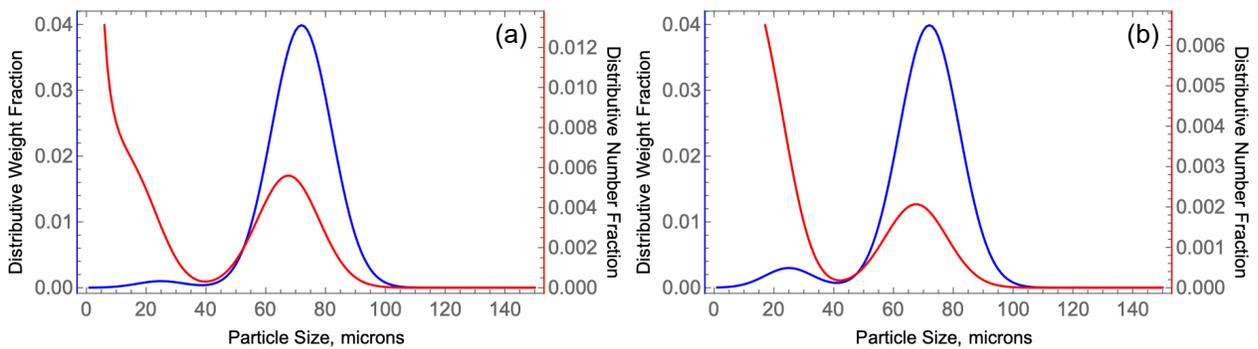
Figure 3: PSDs in terms of weight and number fractions for a Geldart Group A material with (a) 2 wt% and (b) 6 wt% fines ( $d_p < 44$  microns).
