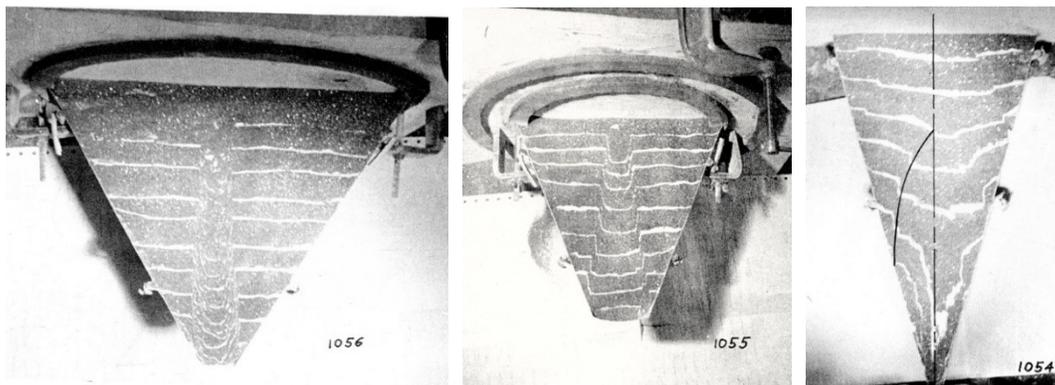
**Figure 2. Early experiments to confirm radial stress in hopper flow**
