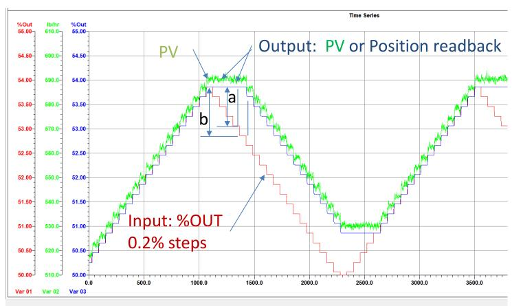
An *input* reversal of amount "a" did not initiate a change in the *output*, but a larger reversal of "b" did initiate a change in the *output*. For dead band, the input change does not change the output.
