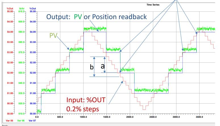
An *input* change in the same direction of amount "a" did not initiate a change in the *output*, but a larger reversal of "b" did initiate a change in the *output*. For **resolution**, the input change does change the output.
