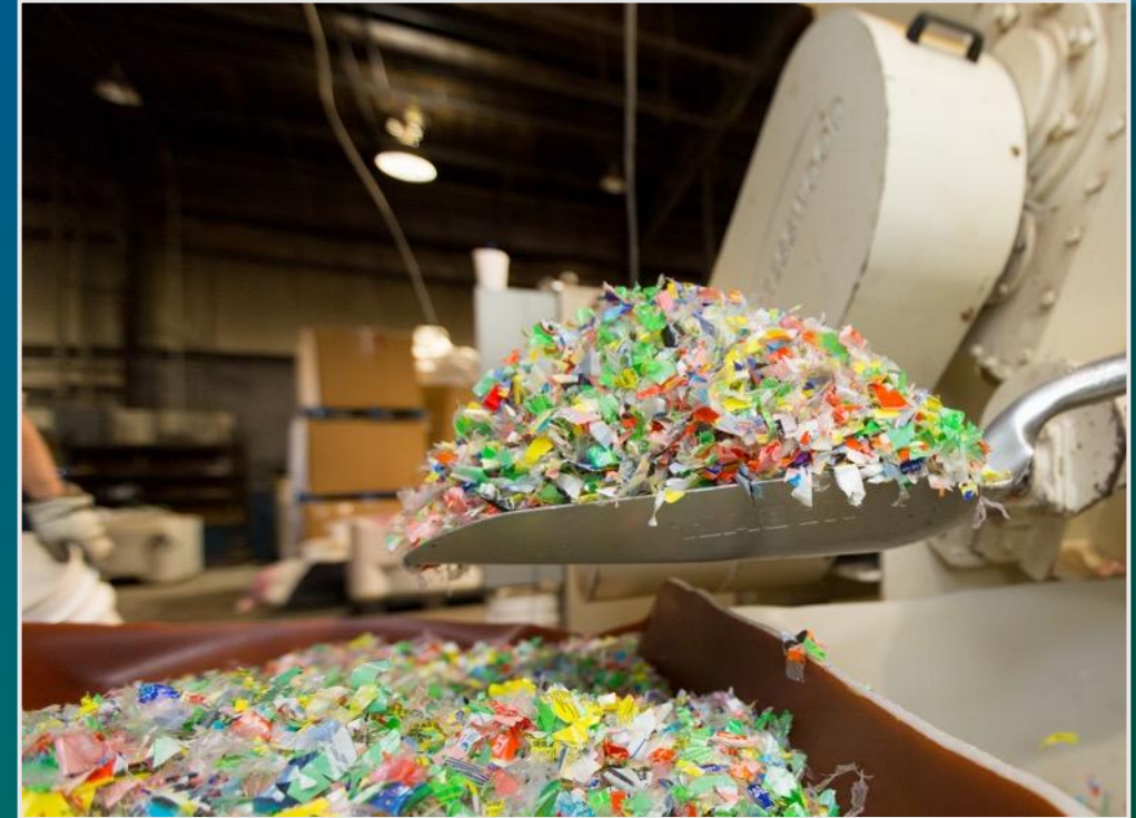
Shredded plastic feedstock at New Hope Energy's facility in Texas, USA
