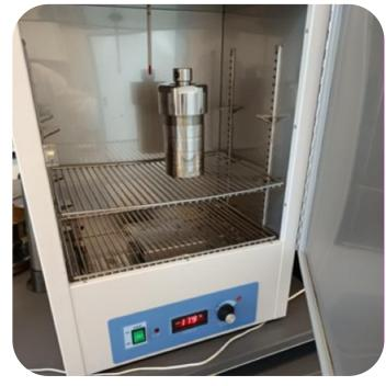
The autoclave is put inside oven for desired temperature and time
