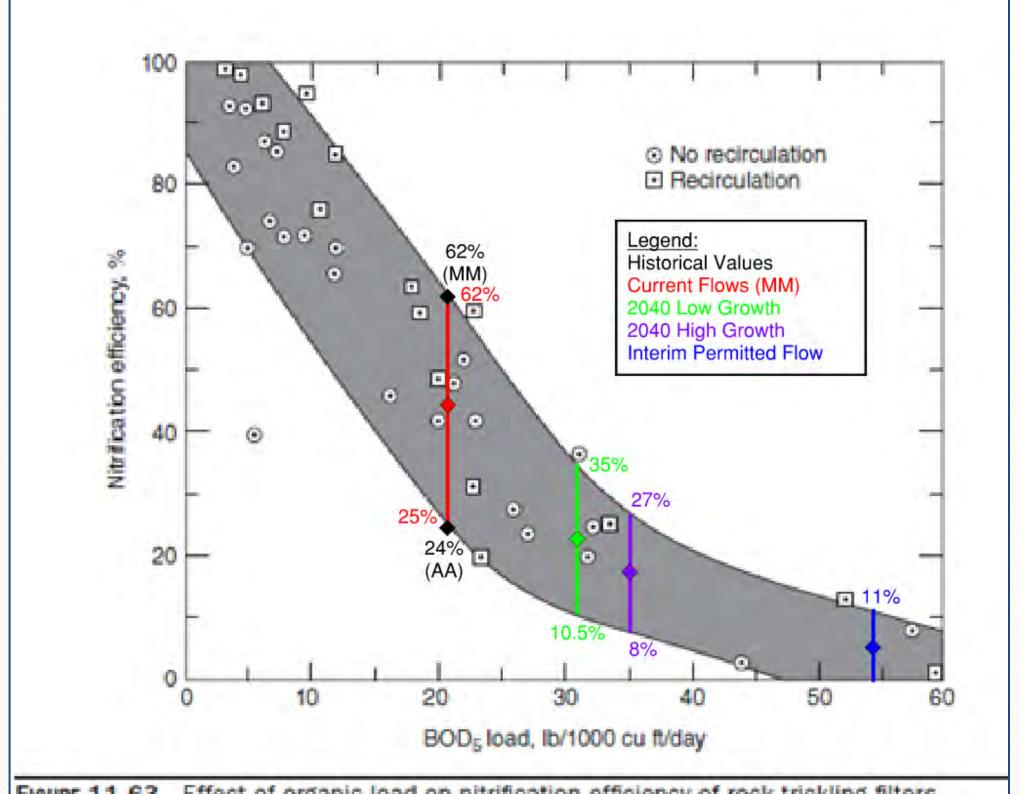
FIGURE 11.63 Effect of organic load on nitrification efficiency of rock trickling filters (lb/d/1000 cu ft  $\times$  0.016 02 = kg/m<sup>3</sup>·d),
