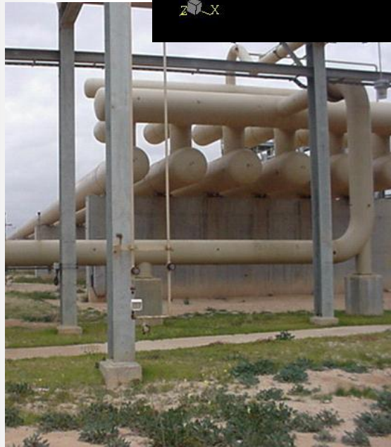
Slug catcher at the Hannibal terminal, U.K.
