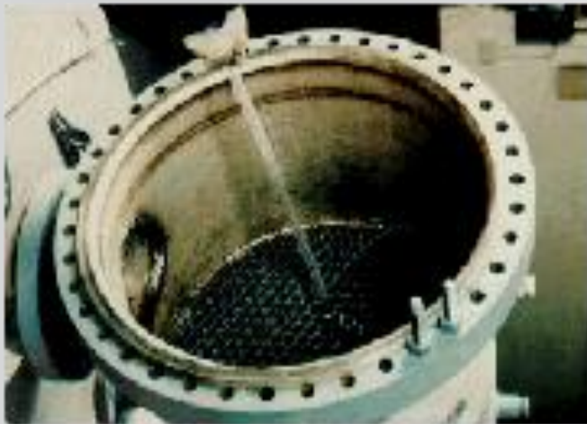
Under-performing, 324 tube, heat exchanger
