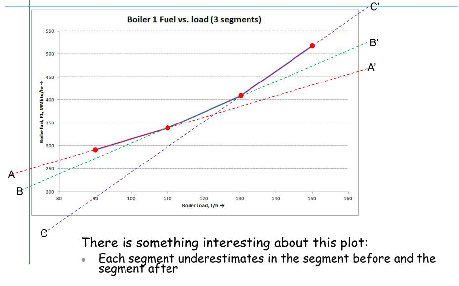
This fact could/should be used in efficient modeling of the boiler
