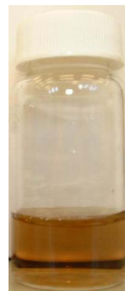
4-nm Pd-on-Au NPs (~6 wt% Pd)
