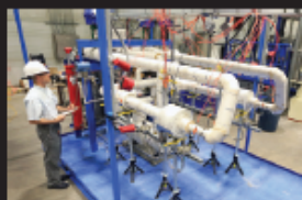
One of three fouling research rigs
