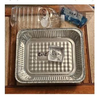
c. Begin adding weight pellets very carefully inside the center of the foil boat. Continue adding weight pellets until the foil boat sinks into the water and fails to float.
