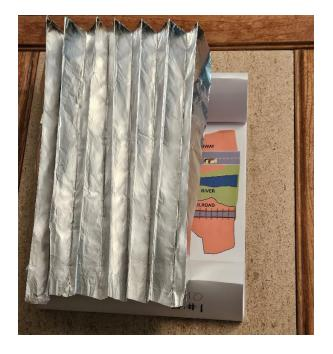
g. Next place the white paper deck on top of the foil Zig-Zag support structure. This deck will support the load of the weight pellets with the foil structure beneath.
