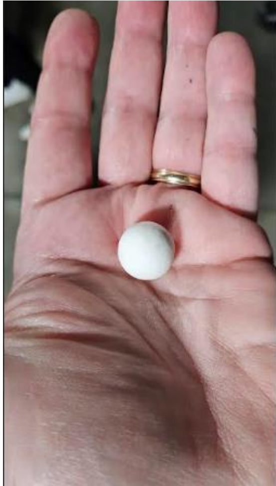
Ceramic Beads used in metals heat treating process
