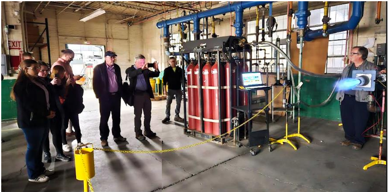
Burner flame demonstration comparing Hydrogen, Natural Gas, and air mixtures
