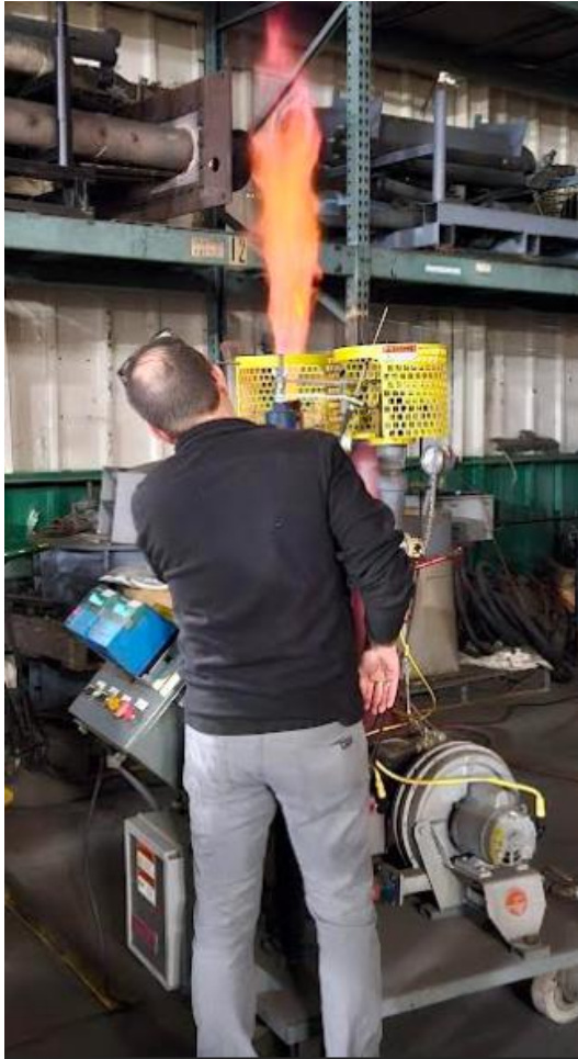
Burner flame demonstration comparing Hydrogen, Natural Gas, and air mixtures
