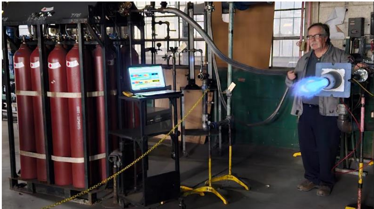
Burner flame demonstration comparing Hydrogen, Natural Gas, and air mixtures
