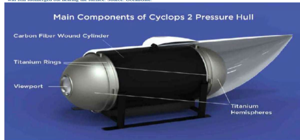
Figure 155: Main components of the CYCLOPS II (TITAN) pressure hull. Source: OceanGate.
