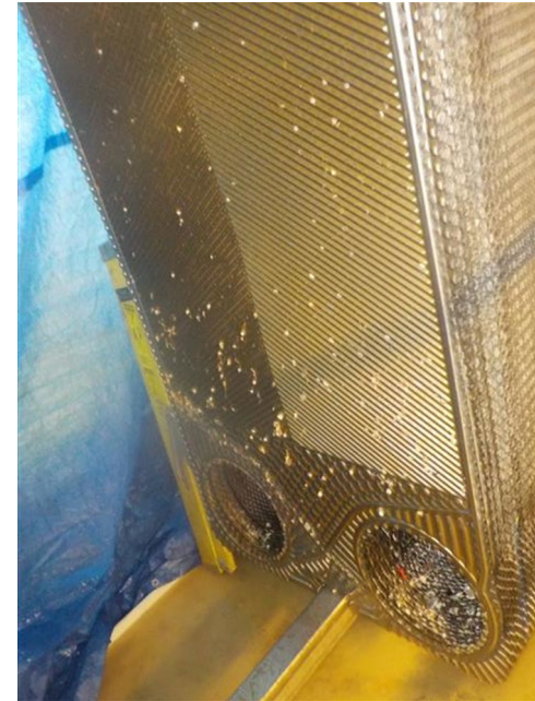
Forward engine cooler No biological or mineral fouling
