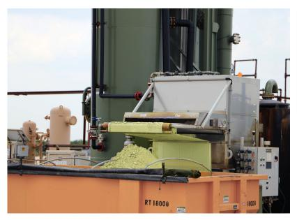
Elemental Sulfur is filtered and water washed by an automated filter press and dumped in a roll-off box, hauled to landfill or reused for agricultural soil amendment.
