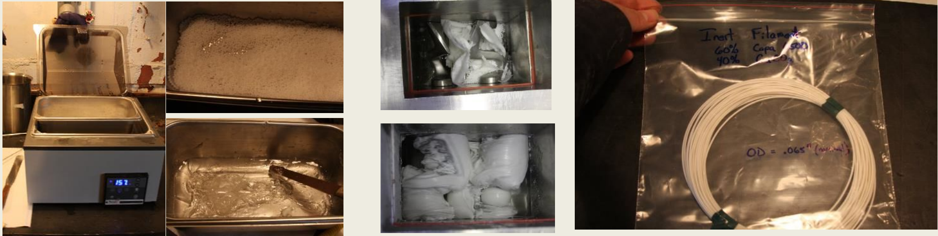
Melting Experiment (Left Section), Mixing (Middle Section), Extruded Filament (Right)
