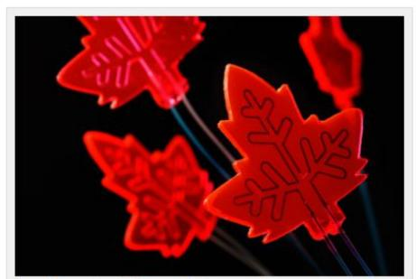
Leaf-Inspired Microphotoreactors Figure 1. The amount of light captured by the microphotoreactors is visible, lit up bright red. As liquid is pumped through thin channels or "veins" in the leaves, light causes the reactions. *Source: Bart van Overbeeke*. The leaf, made from silicone rubber, can operate in diffuse light. "It can be easily cleaned with some solvent and subsequently reused," says Noel.
