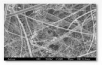
Vapor grown carbon fibers (VGCF) entrapped in 2.4 µm glass-MFM
