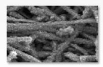
Vapor grown carbon nano-fibers (VGCNF) grown on 1.5 µm Ni-MFM
