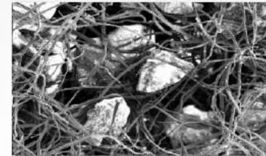
180-250 μm g-Al<sub>2</sub>O<sub>3</sub> entrapped in 8mm SS Fibers
