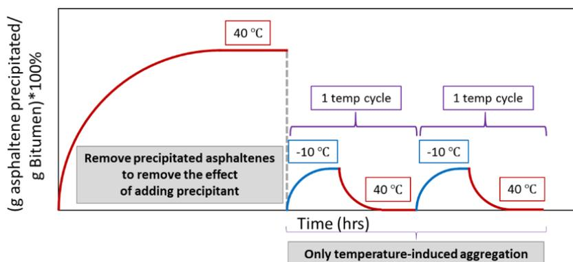
Asphaltenes are the heaviest oil fraction that can destabilize due to changes of pressure, temperature, and/or composition, causing reduction in oil production and fouling issues.
