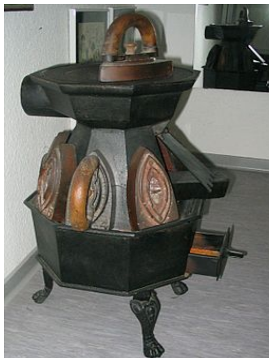
FIGURE 1 ONE OF MANY WAYS TO SPEED UP THE TEDIOUS IRONING PROCESS WAS TO ALWAYS HAVE AN IRON ON THE FIRE, READY TO USE, WHEN THE ONE IN USE COOLED OFF. [PHOTO BY KUERSCHNER, 2008 VIA WIKIMEDIA COMMONS]
