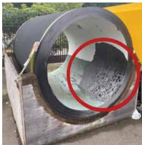
◀ Figure 6. A large crack in the internal hull surface of Version 1's (V1's) carbon fiber hull could have alerted engineers to inherent flaws in their design strategy (1).
