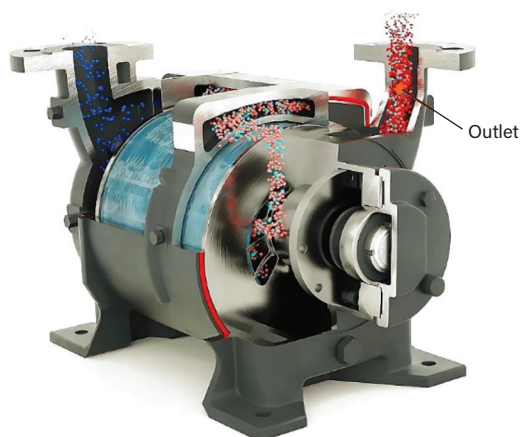
▲ Figure 1. This cross-section of a liquid ring vacuum pump illustrates how process gas is trapped and compressed between the liquid ring and rotating impeller. Depicted is a model from the DOLPHIN series by Busch.
