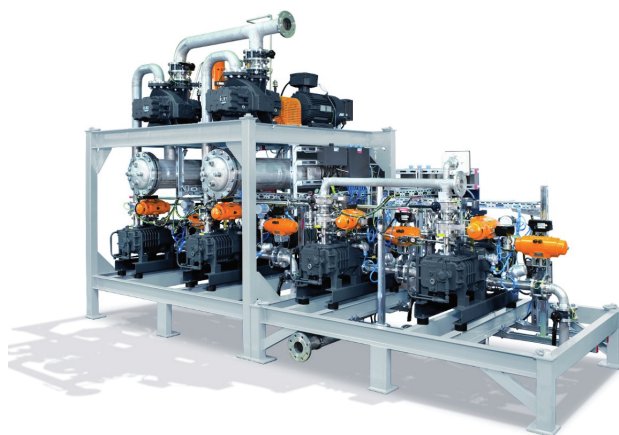
▲ Figure 4. Vacuum systems can be configured in modular arrangements to meet space constraints. A gas cooler is integrated between stages to prevent overheating and reduce the temperature of the process gas before it enters the screw vacuum pumps. This tailored configuration ensures efficient multi-stage compression and reliable operation in demanding chemical environments. The image shows a custom-engineered vacuum system from Busch Vacuum Solutions with PANDA and PUMA vacuum boosters as the first stage and COBRA screw vacuum pumps as backing pumps.
