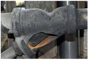
▲ A cast iron Y-strainer failed during operation and released flammable isobutylene. See the U.S. Chemical Safety and Hazard Investigation Board (CSB) Report No. 2019-02-I-TX for more detail.
