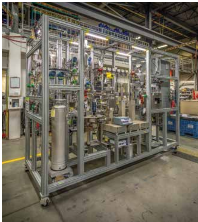
▲ Figure 9. Using an aluminum frame instead of a steel or stainless steel frame for a modular unit can reduce manufacturing costs and weight while maintaining a high degree of corrosion resistance and recyclability.
