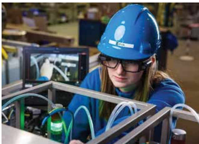
▲ Figure 6. Factory acceptance testing can be carried out remotely via a direct video link.
