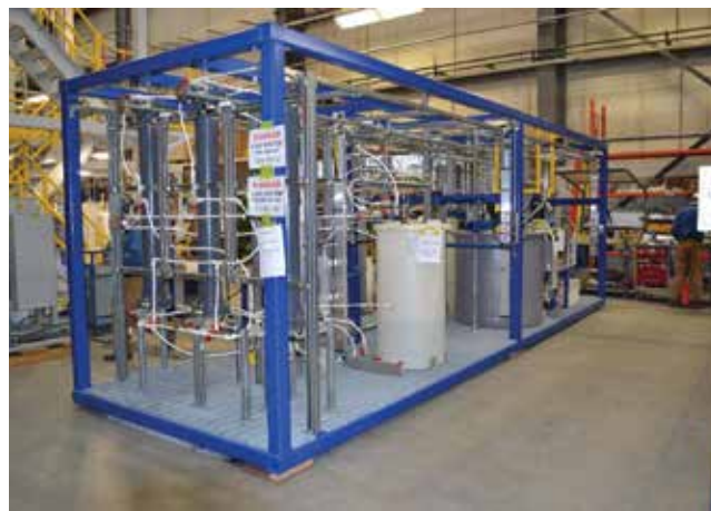
▲ Figure 8. Using plastic vessels and tubing, as shown in this lithium extraction pilot plant, reduces weight and manufacturing costs.
