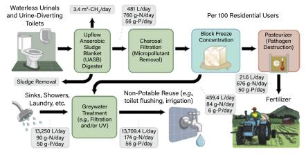
Brightwater Tools' innovative equipment presents an integrated system for nutrient recovery and non-potable water production from residential wastewater. In this flowchart, g-N/day and g-P/day stand for grams of nitrogen or phosphorus per day, respectively.
