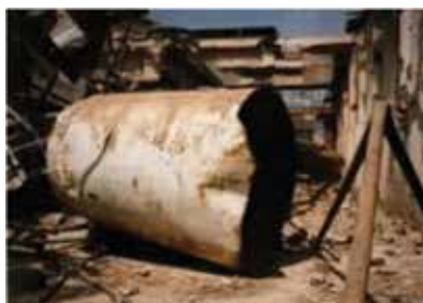
▲ Figure 2. The exploding tank split into two pieces that were propelled in different directions. These images show the front of the tank from view 1 (left), the front of the tank from view 2 (center), and the rear of the tank (right) (1).
