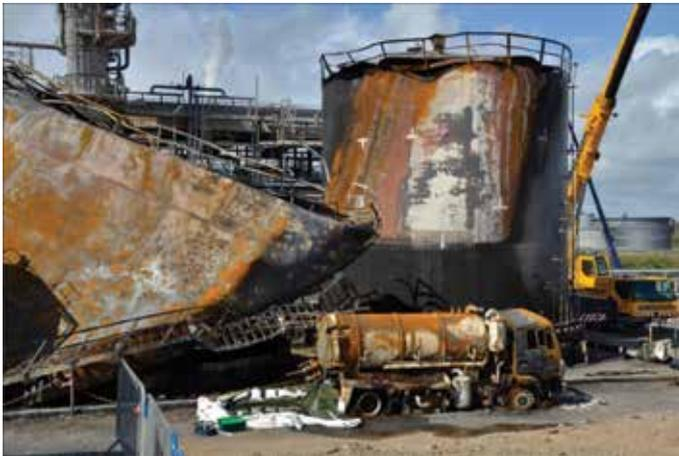
▲ A storage tank at a refinery exploded during a routine cleaning operation. Image courtesy of the U.K. Health and Safety Executive.
