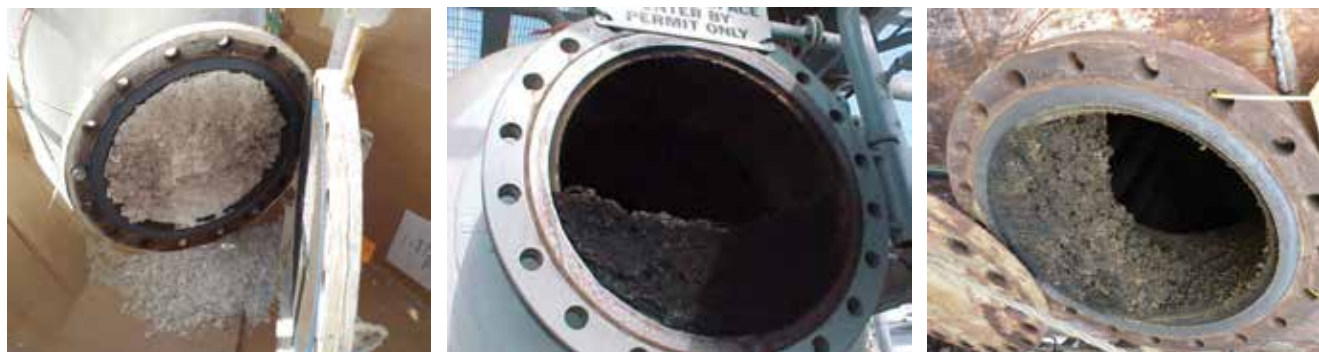
▲ Figure 3. Deep manways are often overlooked stagnant areas where polymer can form.
