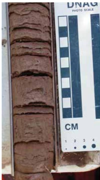
◀ **Figure 2.** A Geoprobe core of varved clay was collected from a former manufacturing site near Hartford, CT, where solvents were released into the ground. The dark horizontal bands are the silty (more permeable) layers, and the thicker, lighter bands are the clayey layers. The cupping around the edges is a remnant of the drilling process.
