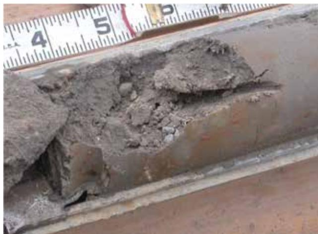
▲ **Figure 1.** A split-spoon core sample of glacial till was collected from a former manufacturing site in Flint, MI. Oil in the subsurface was released from the manufacturing process. Note the mixture of clay, silt, and gravel-sized particles, and that the core is dry.
