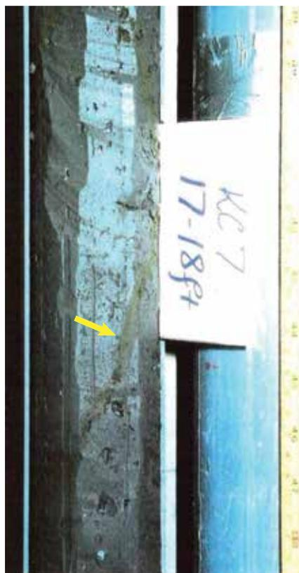
◀ **Figure 5.** This photograph shows a fractured clay core from Essex County, Ontario. The fracture is the reddish slash (at the tip of the yellow arrow) between 17 ft and 18 ft (5.2 m and 5.5 m) below ground level. This core was part of an isotopic investigation of the age distribution of the groundwater in a thick clayey aquitard.
