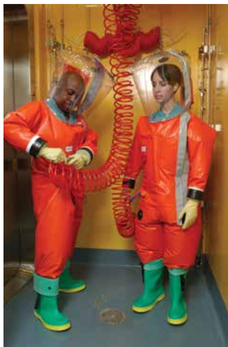
◀ Figure 2. To work in a BSL-4 lab, researchers are required to wear a full-body suit that is connected to an external air supply. Image courtesy of James Gathany and the Centers for Disease Control (CDC).
