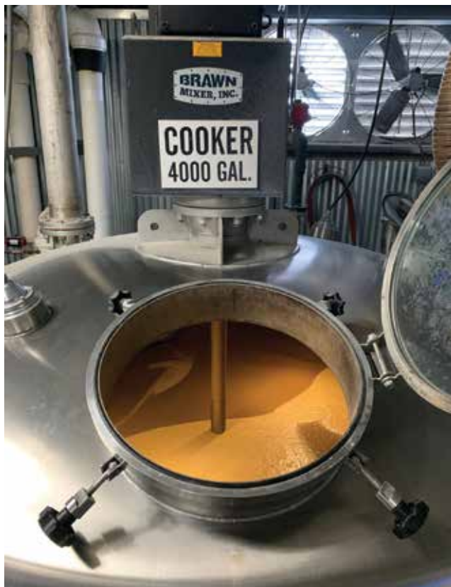
▲ Figure 2. In the mash tun, the grains and water are heated with enzymes that break starches into fermentable sugars.
