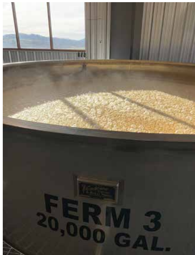
▲ Figure 4. Traditionally, and often still today, fermentation vats are uncovered and open to the environment.
