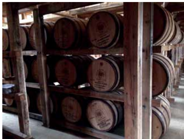
▲ Figure 7. These photos show the outside and inside of a rickhouse that is not temperature controlled. The temperature variations cause the bourbon to expand and contract in the barrel.
