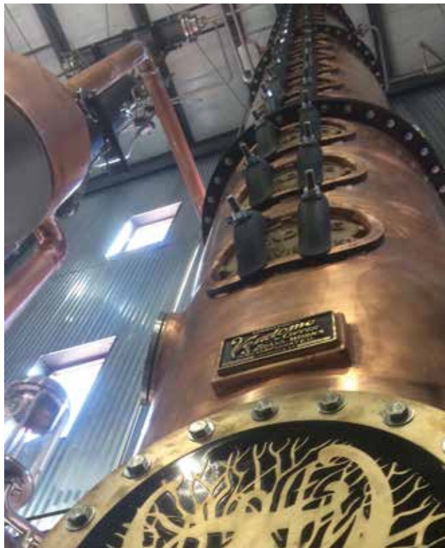
▲ Figure 6. The stills used in bourbon production operate under the same principles as distillation columns used for separations throughout the chemical process industries (CPI). The stills are constructed of copper, which has antimicrobial properties, and reacts with sulfur to form copper sulfate, effectively removing sulfur from the distillate and improving flavor.
